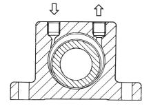
Housing made from extruded aluminium alloy Highly flexible steel guides Cast precision steel roller Special bronze end plates
